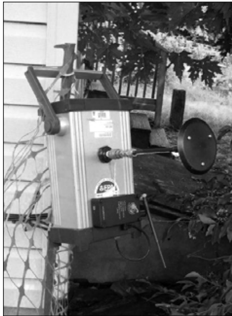
A monitor detects air particles to ensure proper air quality during soil excavation.
